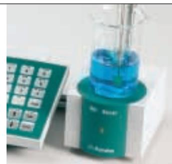
The 804 Ti-Stand with 802 Rod Stirrer offers an alternative way of stirring.
