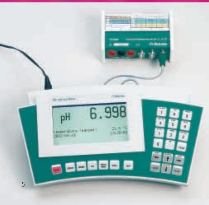
Checking the pH display of the 781 pH/Ion Meter with the 767 Calibrated Reference.
