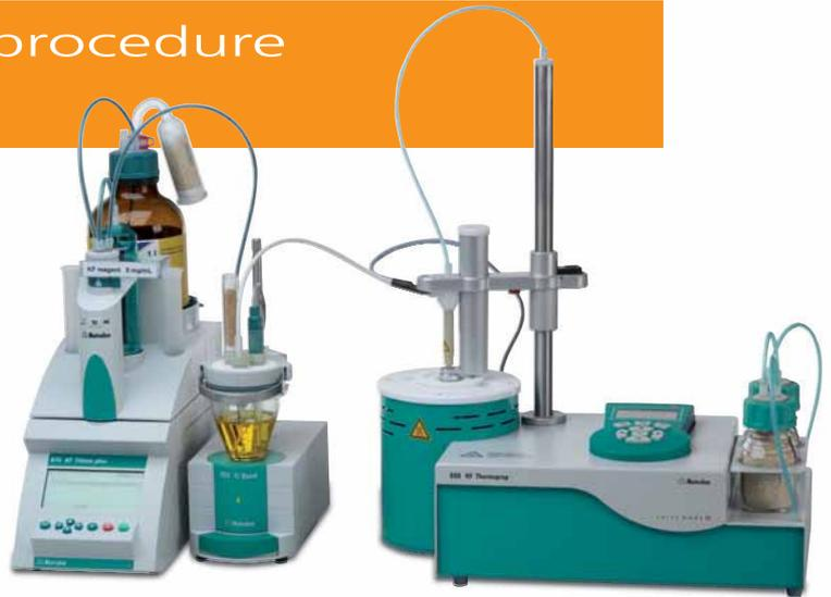
The sample is weighed into a sample vial and hermetically sealed. After the desired temperature has been reached and the titration cell conditioned, the determination is started at the KF coulometer (or KF titrator). The vessel containing the sample to be analyzed is positioned in the oven and the needle inserted through the septum of the sample vial.
